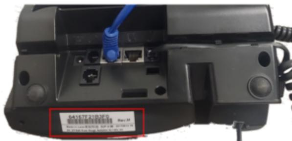
2. Next power off the telephone by removing the power supply or network cable (POE users).
